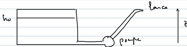
$$\hookrightarrow v_s = Dv \cdot s^{-1} = 4 \frac{Dv}{\pi d_1^2} \gg v_e \approx 0 \quad (L^2 v_0 = 8 v_s)$$
