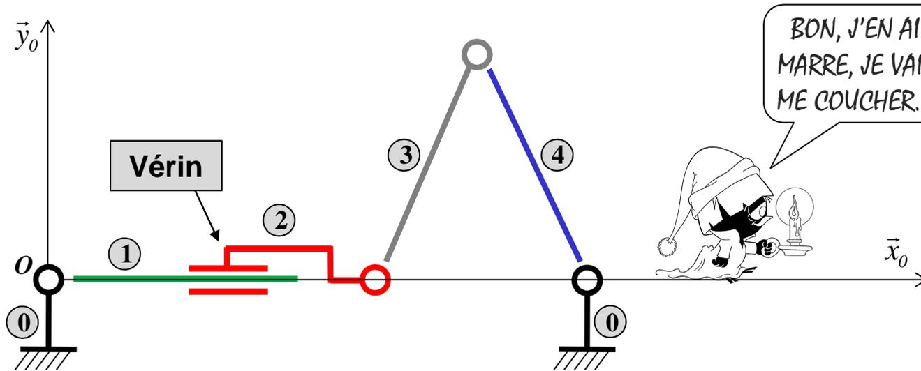
$$\textcircled{1} \quad \{V_{1/0}\}_O = \{V_{1/2}\}_O + \{V_{2/3}\}_O + \{V_{3/0}\}_O$$
