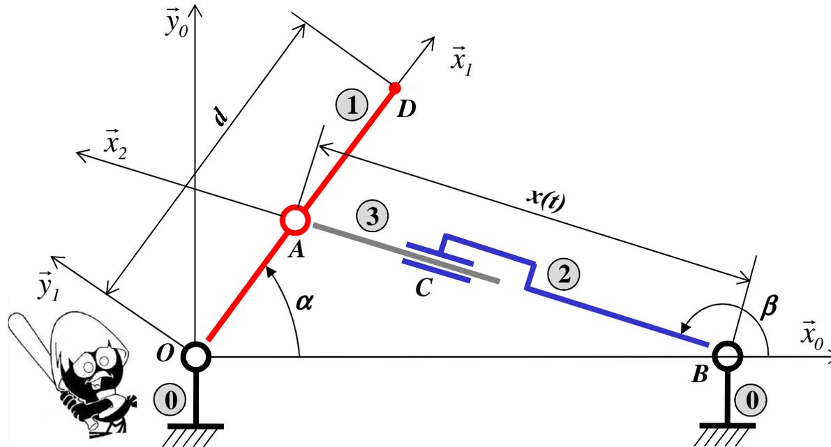
$$\textcircled{1} \quad \{V_{1/0}\}_O = \left\{ \begin{array}{l} \dot{\alpha} \vec{z}_0 \\ \vec{0} \end{array} \right\}_O$$
