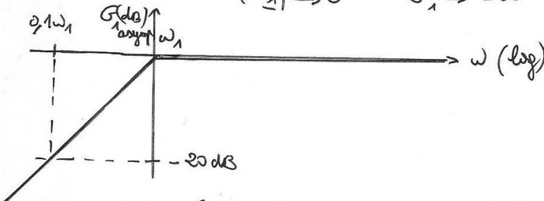
Q.8. A.N.:  $f_1 = \frac{1}{2\pi R_1C_1} = \frac{1}{2\pi \times 10^5 \times 10^{-7}}$
